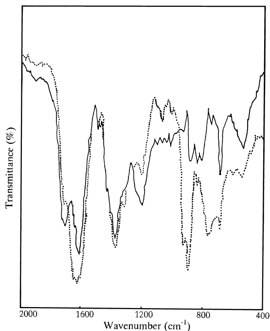
Fig. 1. Infrared spectra of Amberlite IRC748 (—) and IRC748/Mo/aq catalyst (.....).
